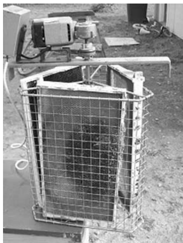
Fig. 21. Inside a motorized tangential extractor
